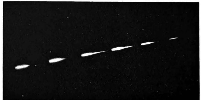
A bright meteor trail recorded at one of the twelve field stations of the Meteor Observation and Recovery Project which is operated by NRC in the prairie provinces. The trail image is chopped 3 times per second by a rotating shutter to provide velocity and deceleration data. This meteor trail is about 25 km long at an altitude of about 90 km. Such meteors very often generate UFO reports.
